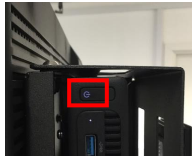
Location of power button, lit when PC is on
